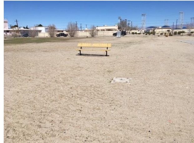
MJH58 – pulverize asphalt court and smooth grade; remove concrete structure & bench; import clean fill dirt; smooth finish grade; no ponding
