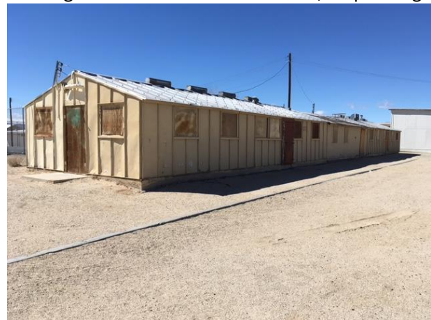
MJH54 – demolish & remove from site metal building, SOG, footings, cut & cap water, sewer & gas 5' from building; remove power pole, bf/compact; import clean fill dirt, smooth finish grade area with adjacent area of MJH 52 (track & field); no ponding in finish grade
