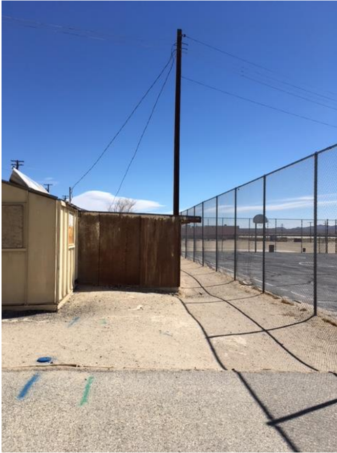
MJH54 – demolish metal & wood building; remove wood power pole; remove abandoned power line back to MJHPE building & disconnect at electrical panel; C.L. fence & basketball court to remain; smooth finish grade, no ponding
